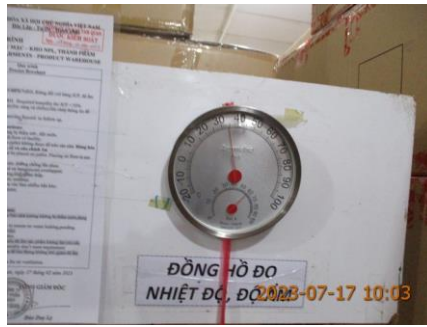
Photo 77) NC#7.3.1: It was noted that 01 temperature and humidity meter at finished good warehouse were not calibrated before use.
