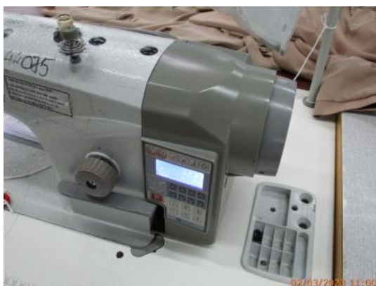
59. Pulley guard was equipped for sewing machine.jpg
